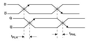
Figure 2. Propagation Delay
