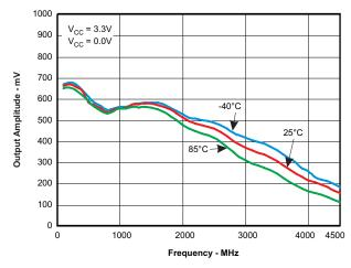
Figure 6. Output Amplitude vs Frequency
