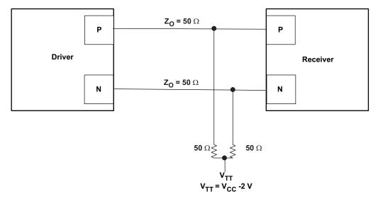
**Figure 1. Typical Termination for Output Driver**
